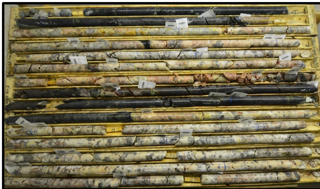
Figure 2. Drill core obtained from hole SL-16-68 showing a portion of the 16m intersection of high quality spodumene-bearing pegmatite.
