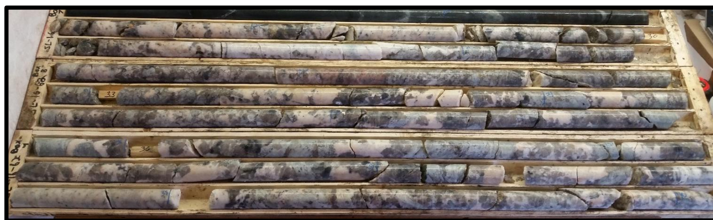
Figure 1. Drill core obtained from drill hole SL-16-62 showing the 11.5m intersection of high quality spodumene-bearing pegmatite.
