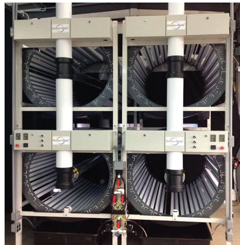
Figure 3: Roto-Gro 420 units stacked in 2 x 2 configuration
