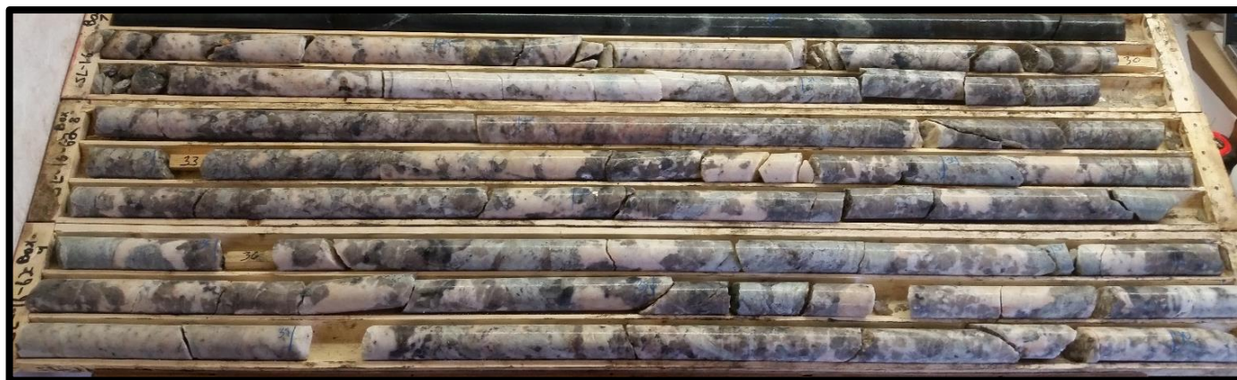
Figure 1. Drill core obtained from drill hole SL-16-62 showing the 11.5m intersection of high quality spodumene-bearing pegmatite.
