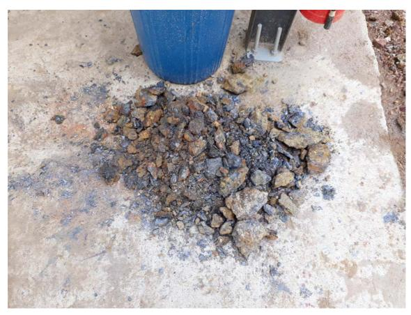
Figure 4: Weathered vein graphite extracted from Shaft J as it is being sunk
