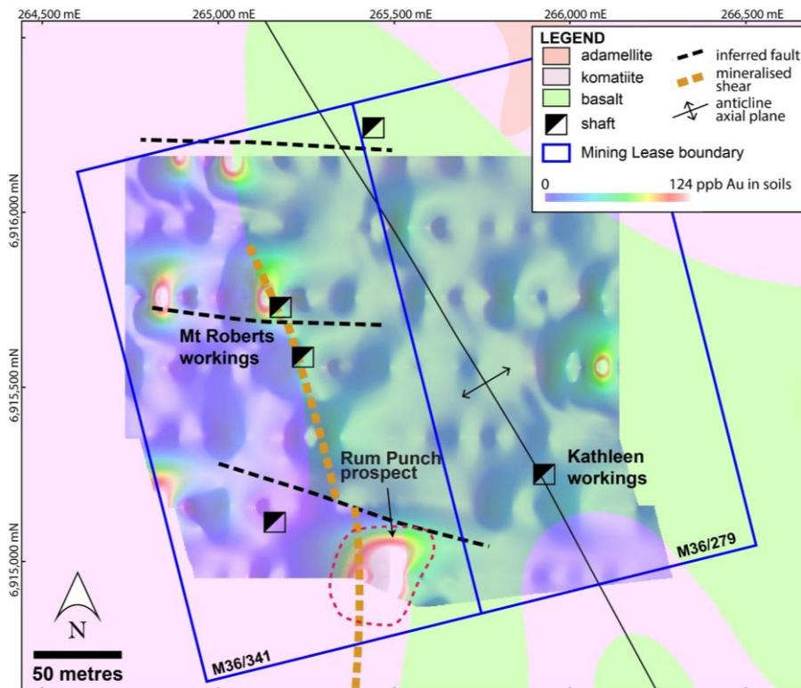
Figure 4. Geology of the Mt Roberts-Cottee Project area, showing the distribution of historical workings, structural interpretation and gold anomalism in historical soil samples. Historical soil results were gridded using a minimum curvature algorithm and cell size of 2.5m<sup>2</sup>.
