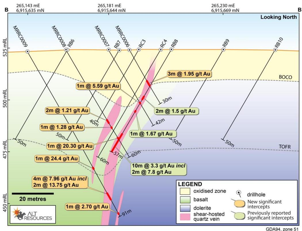
Figure 5. Cross-section showing significant mineralisation in Alt Resources drillholes MRRC0006, 0007, 0008 and 0009. Significant intercepts in historical drillhole RB8 are also shown. The interpretation of new data reveals that historical drilling was likely parallel to the orientation of the structure. RB8 drilled down-dip through the mineralised shear zone, whereas surrounding drillholes intersected no mineralisation.
