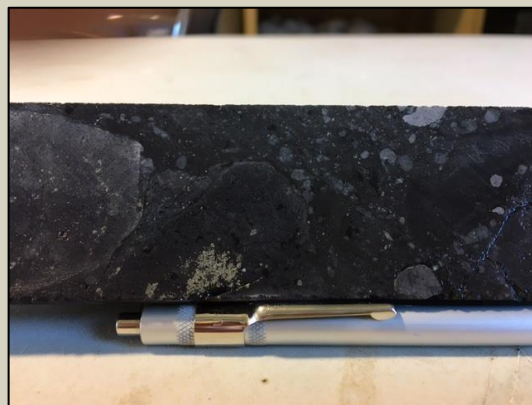
Photo 2. Polymict breccia with multiple phases of sulphide mineralisation.
