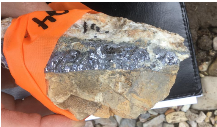
Figure 3: LEFT A veinlet with coarse galena (lead sulphide) and sphalerite (zinc sulphide) occurring with barite along the margin of one of the large EW veins. There are innumerable such veinlets that appear to be concentrated near the Callancocha Structure (Figures 4 & 6).
