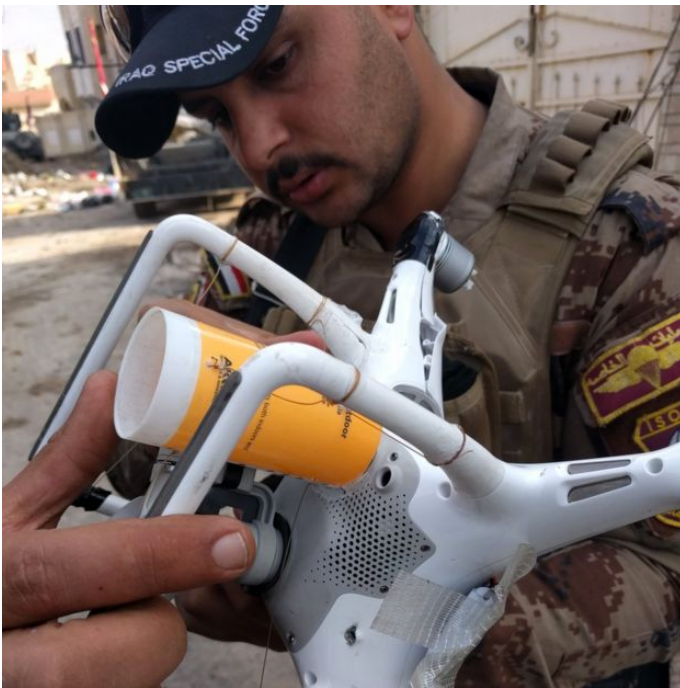
Image: Basic cup holding mechanism for a grenade on a captured ISIS drone 2
