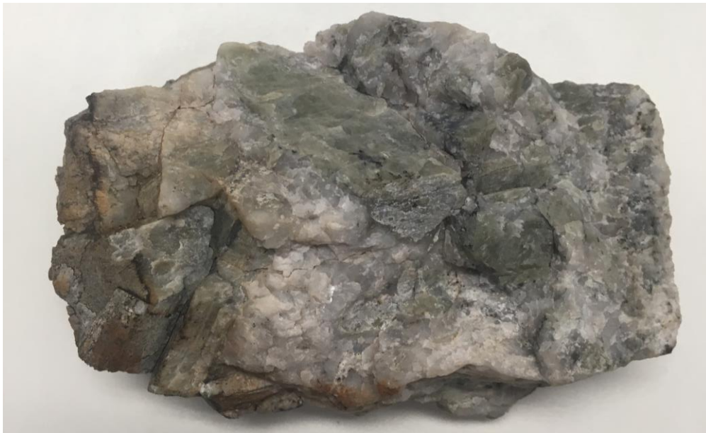
Figure 1. Photo of spodumene bearing pegmatite taken from the surface at Atomic Three, directly above the pegmatite intercept in MERC0002. The sample is approximately 8cm long
