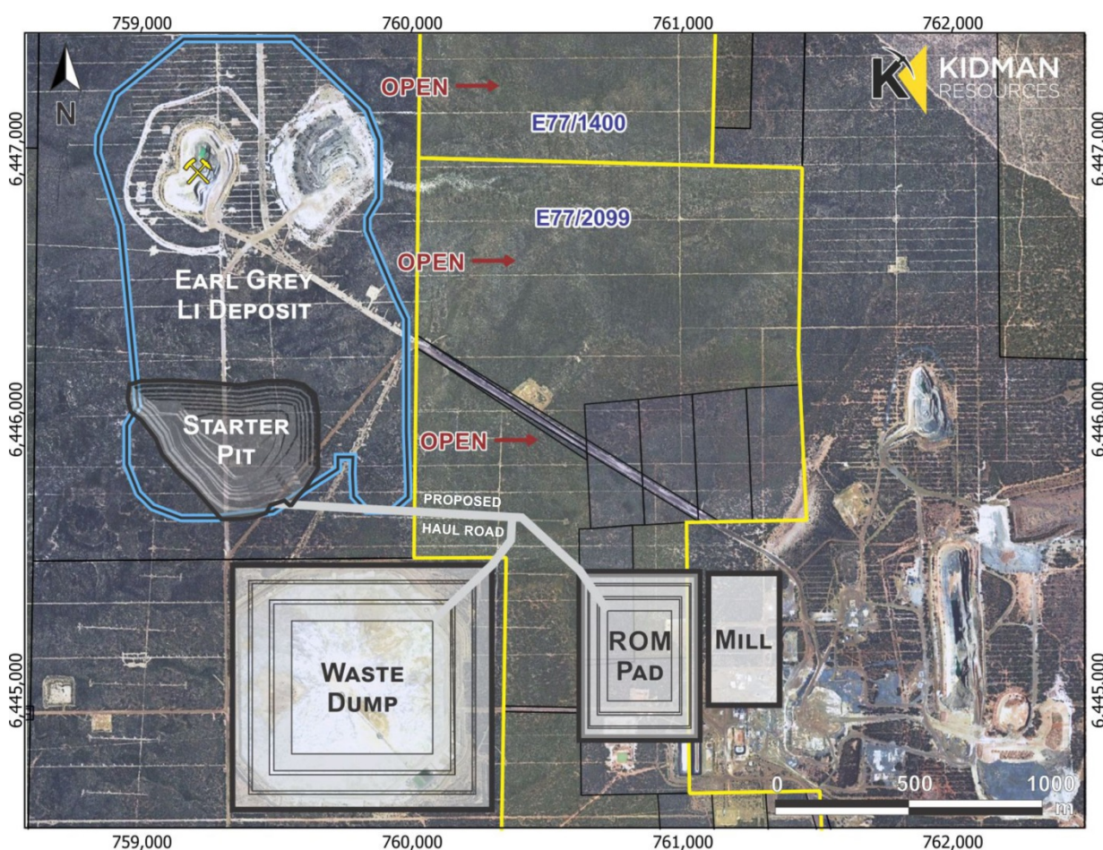
Figure 1: Conceptual site layout and proximity of Earl Grey Lithium Deposit to newly acquired tenements.
