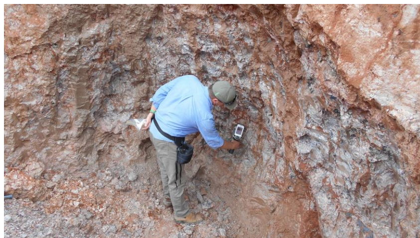
Handheld XRF analysis at Kasombo 6
