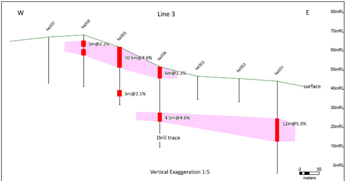
Figure 6. NE Sector cross section, Line 3 mineralised intercepts (3m @ 2% HM cut off)
