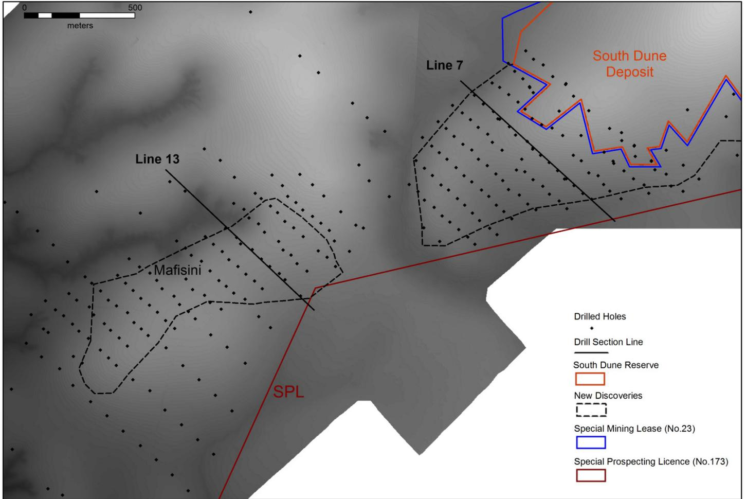
Figure 2. Kwale South Dune Deposit extension and Mafisini Deposit on LIDAR topography
