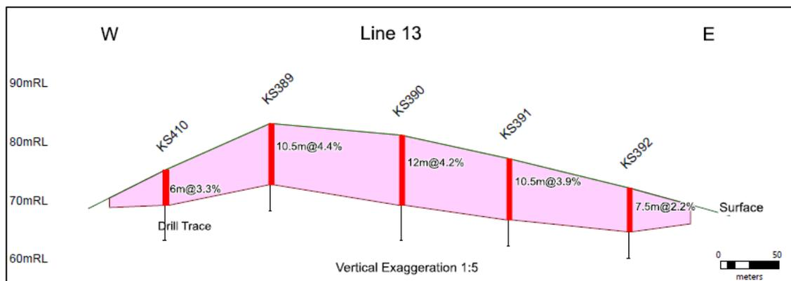
Figure 4. Mafisini Deposit cross section: Line 13 mineralised intercepts (3m @ 2% HM bottom cut off)
