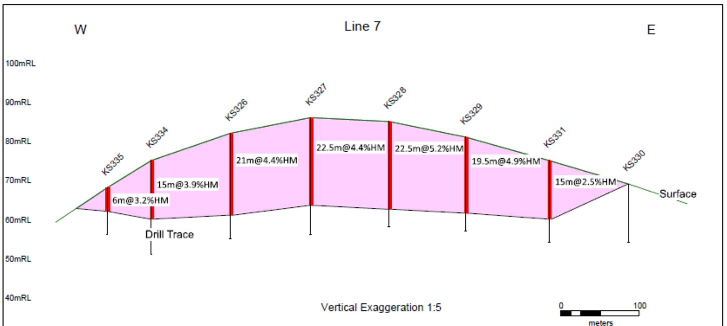
Figure 3. Kwale South Dune Deposit extension cross section: Line 7 mineralised intercepts (3m @ 2% HM bottom cut off)
