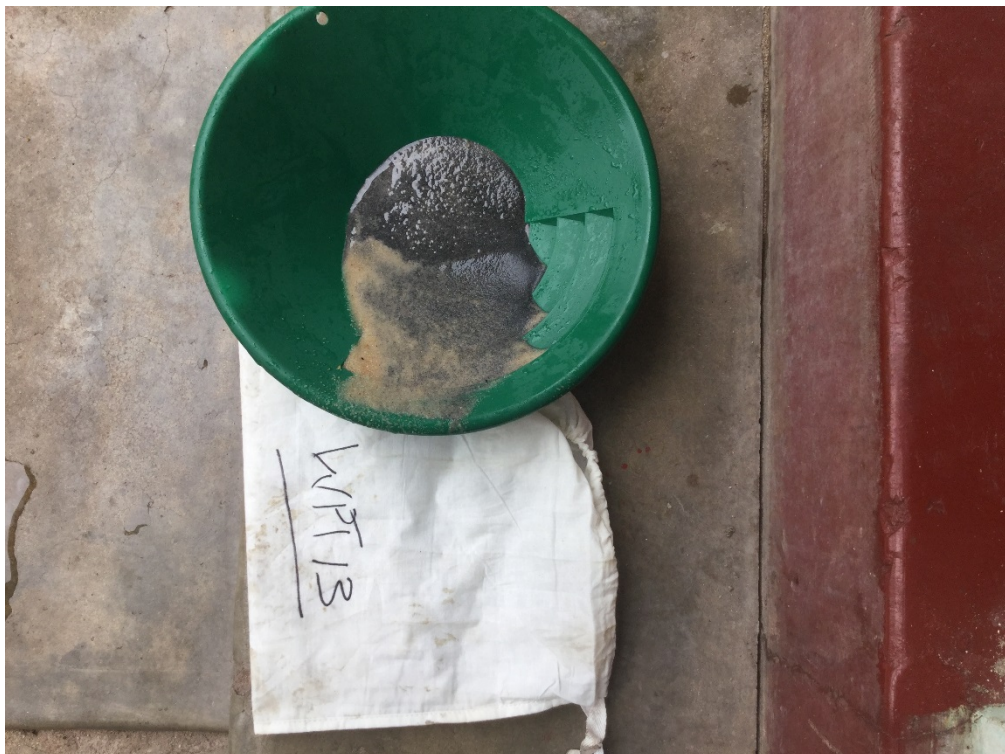
Figure 3 Concentrate of heavy minerals panned from a ~2kg sample from 450m inland at location HG2 in Figure 1.
