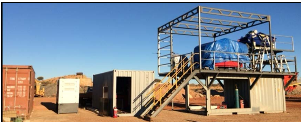
Figure 1: The Ore Sorting Platform, Compressor Module and Generator
