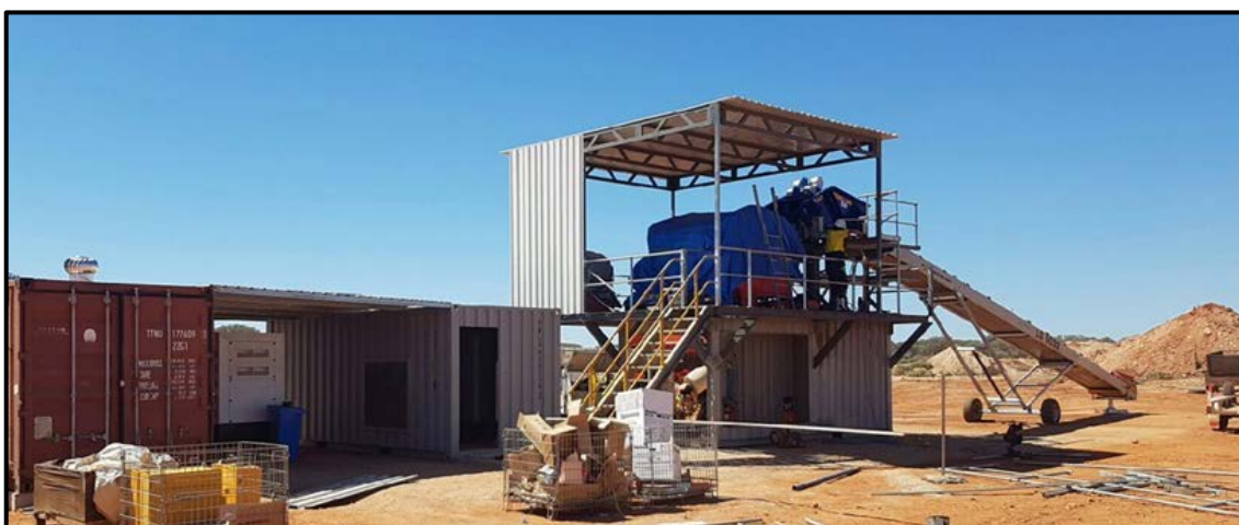
Figure 2: Ore Sorting Platform with feed conveyor and roofing installed.
