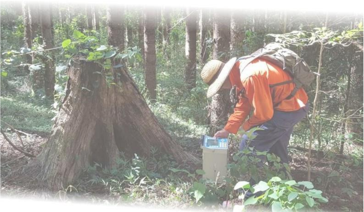
Figure 5. Undertaking gravity surveys at Mary Valley Project
