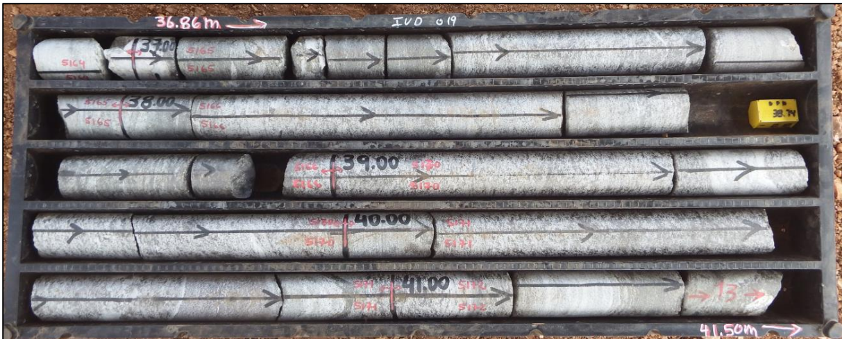
Figure 5: Example core photograph of graphitic gneiss (approximately 6% TGC) between 36.86 and 41.5 m downhole in IVD019
