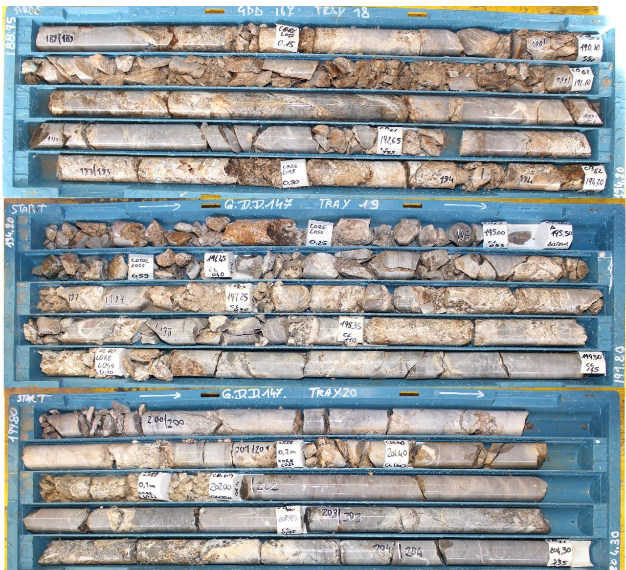
Figure 2: GDD147 intersection containing the zinc and lead oxide minerals (the more friable white, yellow-brown sections) interlayered with grey Breno limestone
