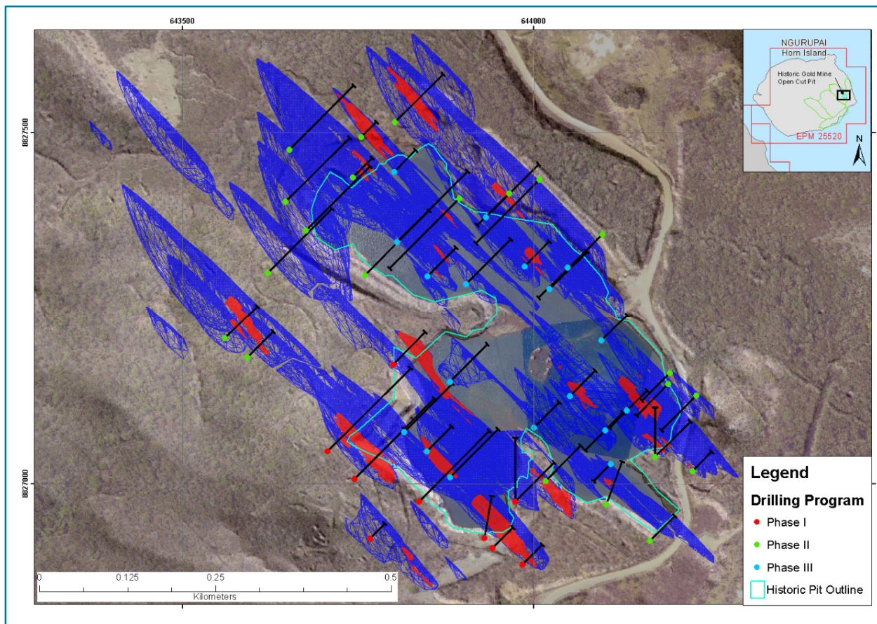
Figure 1 Surface projection of upgraded Exploration Target* - Horn Island Pit Prospect (blue polygon represent 0.5g/t Au cut-off and red polygons represent 5g/t Au cut-off), with planned drilling program phase I to phase III.
