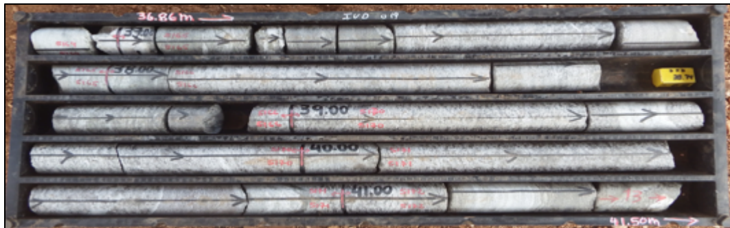
Core photograph of graphitic gneiss (approximately 6% TGC) between 36.86 and 41.5 m downhole in IVD019
