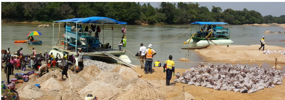
Figure 4. Photo showing two (of three) newly-built dredge units, in operation at the Gbinima locality, Sewa River. Note stock-piled bags containing screened gravel after passing through on-board trommel. The sand overburden has been stockpiled as a community initiative, to allow villagers to pan it for gold (at left).
