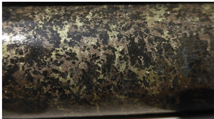
Figure 3 – Close-up of matrix textured sulphides in NQ core 218m AKD017 showing chalcopyrite (Cu), pyrrhotite (Fe) and pentlandite (Ni)
