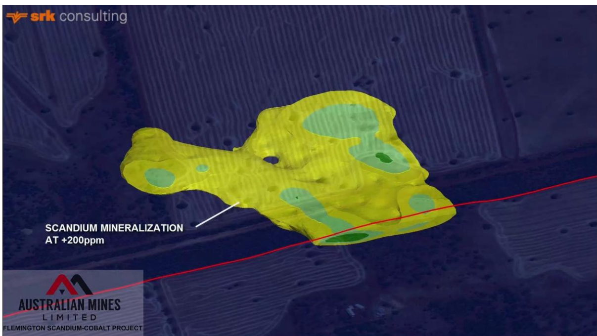
Figure 2: Outline of the scandium ore body at Flemington using a 200 ppm (grams per tonne) lower cut. For scale, the ore body is approximately 500 metres wide and 600 metres long, and terminates to the south at the tenement boundary with Clean TeQ. (Tenement boundary shown as red line)
