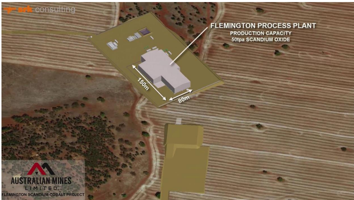
Figure 5: Schematic image of the proposed processing plant footprint at Flemington. Note that the entire processing operation is housed within a modest sized building, which is designed to minimize any potential impacts of visual amenity, noise and dust.
