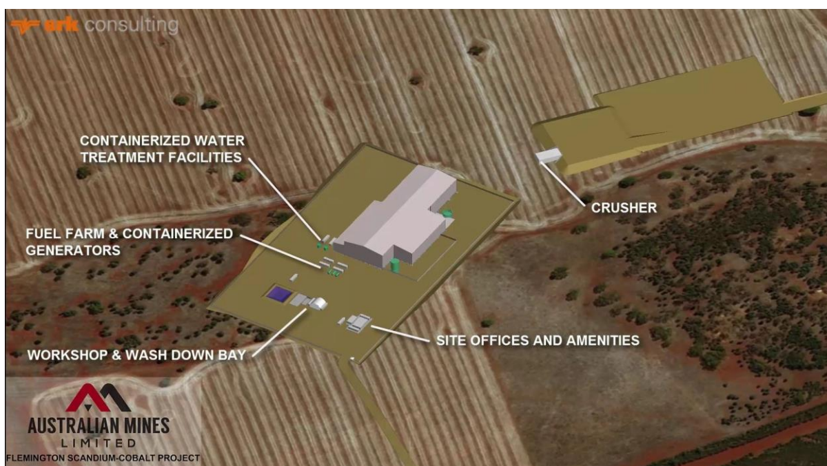
Figure 4: Schematic image showing the proposed footprint of the infrastructure at the Flemington mining operation.
