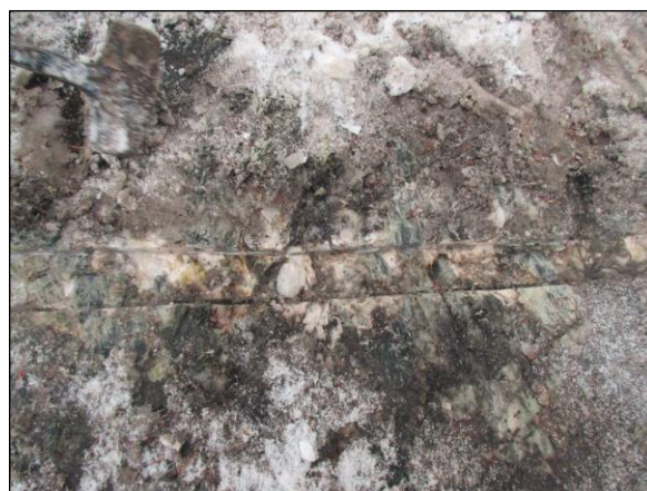
Figure 6: Sample assaying 3.55% Li 2 O in drill target zone from CH16-03
