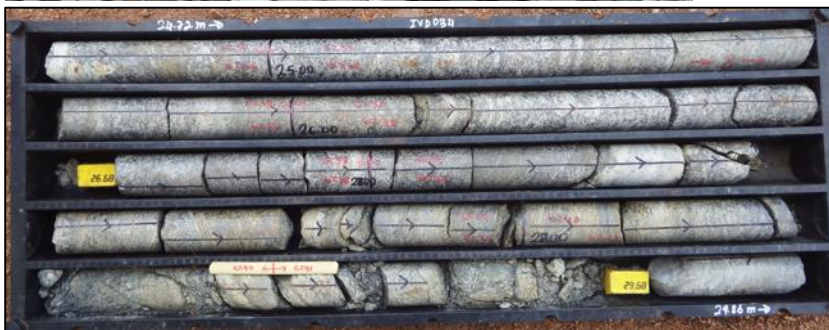
Core samples from T12 IVD034 showing coarse-grained flake graphite in tonalitic gneiss.
