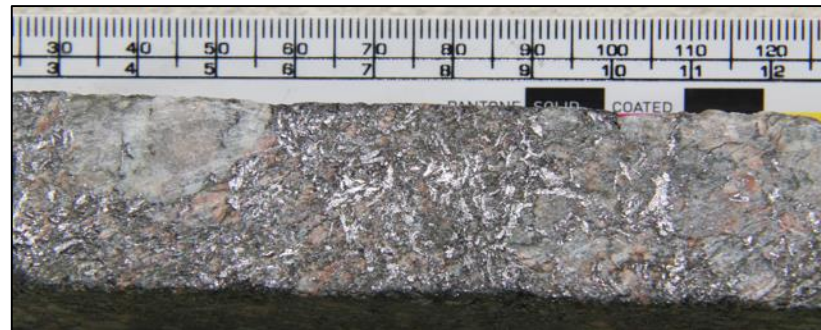
Coarse-grained graphite flakes in gneiss at approximately 58.5 m downhole in IVD034
