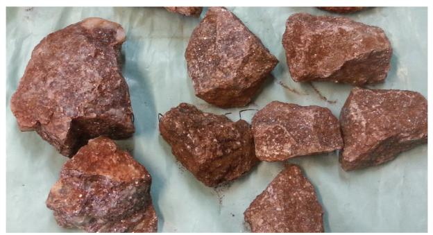
Photograph 1: Crushed Lepidolite mineralisation from the Pioneer Dome in preparation for the L-Max® test programme
