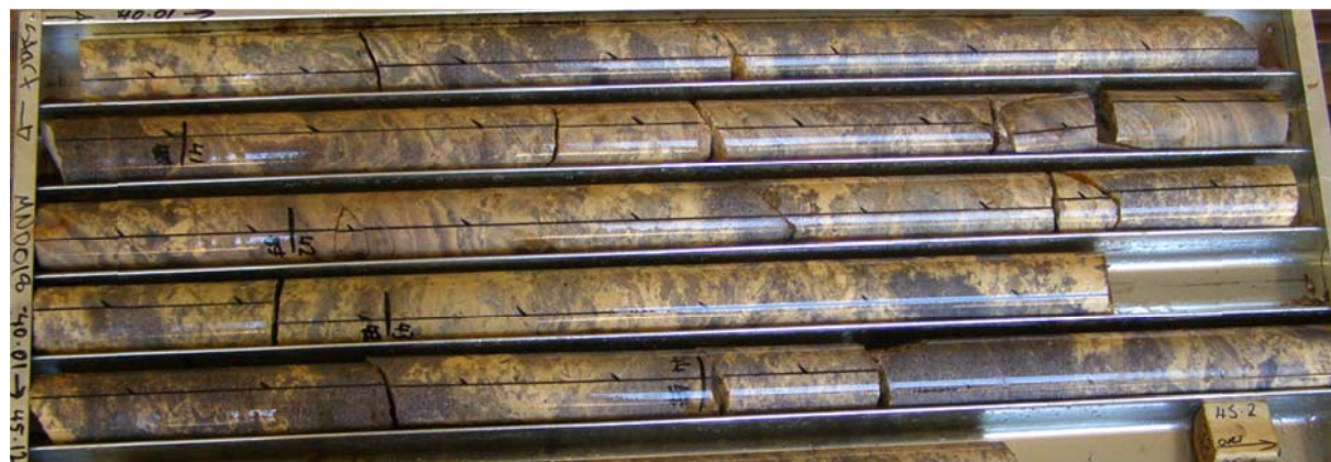
Figure 1 – Diamond core from MND018 showing zone of purple coloured lepidolite. Assaying of this zone returned the highest assay result of 2.14% Li 2 O from 43.36m to 44m. Photo shows diamond core from 40.01m to 45.12m.
