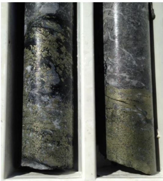
Drill core CCD03 – semi-massive chalcopyrite bands. Contain only very minor pyrite
