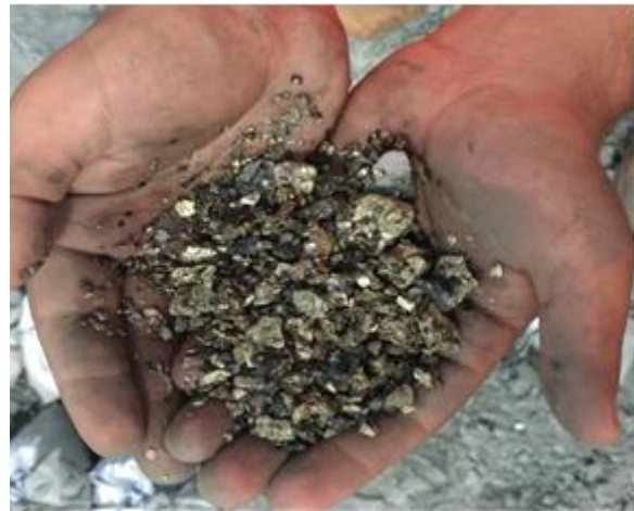
Figure 3: Massive Sulphide Chalcopyrite (primary copper mineral)
