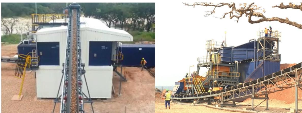
New XRT large diamond recovery and new sorting house (left) and new wet front-end installed at the 150 tonne per hour Lulo diamond plant during 2016
