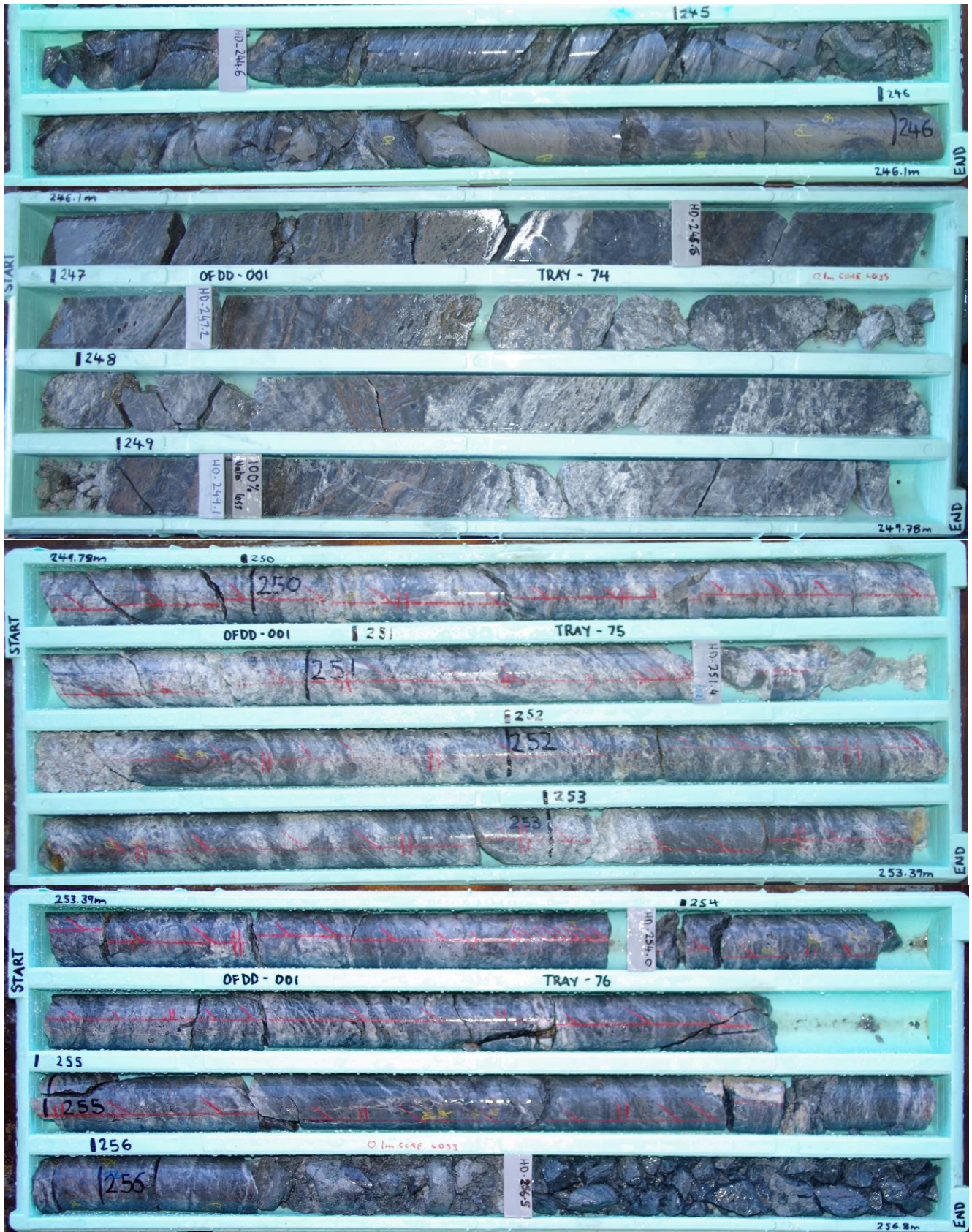
Figure 4: Overflow Prospect diamond drill hole core (OFDD001: 244.5 – 256.8m); upper crustiform vuggy quartz vein dominated mineralised zone showing banded pyrite-sphalerite mineralisation within strongly sheared, silica-sericite-kaolinite altered fine grained calcareous sediments.
