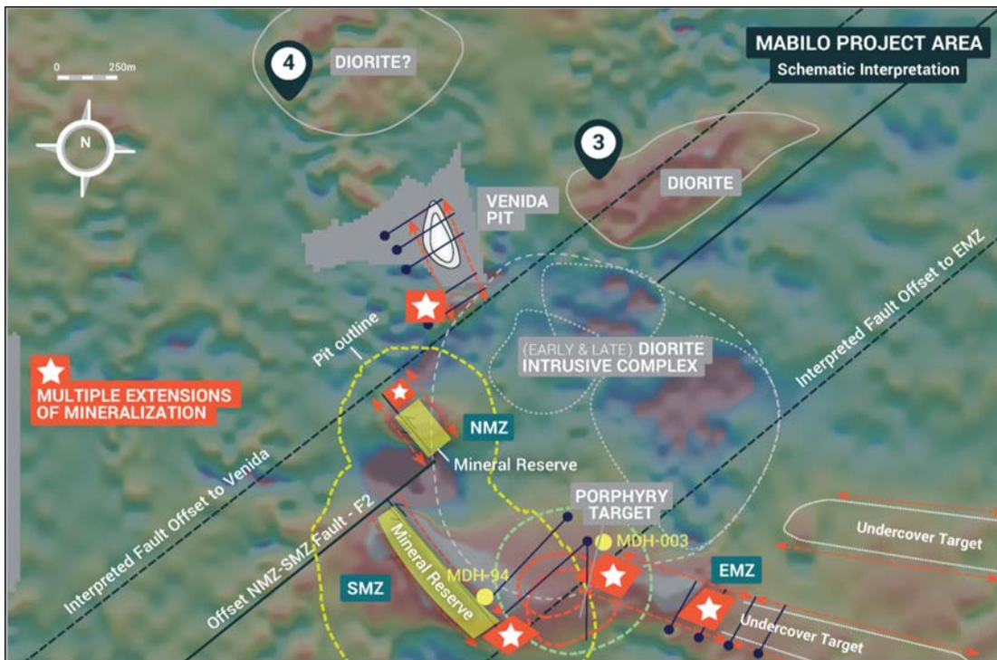
Figure 2 - RTP ground magnetic image with modelled South, North and East magnetic bodies, showing exploration upside targets.
