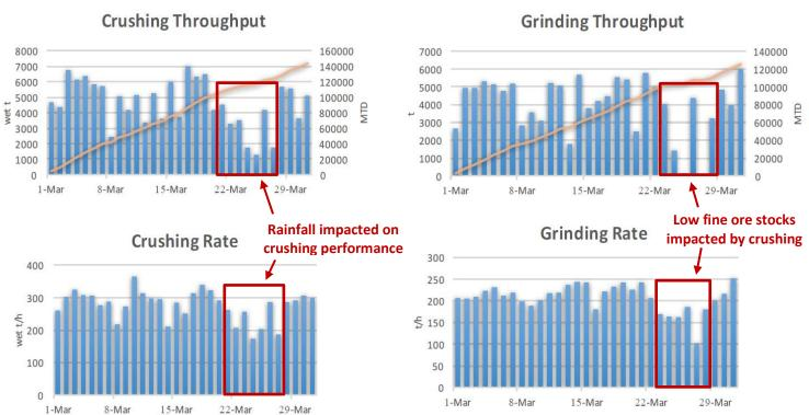
**Grinding Circuit** – Milled throughput has improved every month since commissioning. In the six weeks prior to the rain event, the grinding circuit has operated at an average throughput rate of 4,800 tonnes per day being 103% of nameplate design with a maximum up to 5,800tpd. Weather impact on the
