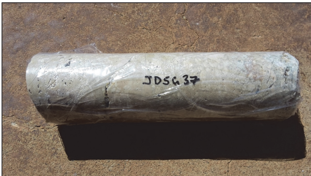
Figure 3 A vuggy and breccia-textured siltstone of JDD004 (JDSG37: 14.73 – 15.00 metres). The sample had a wet SG of 2.18 g/cm 3 .
