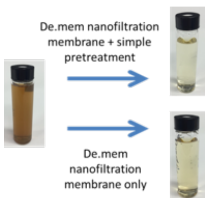
DEMONSTRATION OF DE.MEM NANOFILTRATION MEMBRANE ON PALM OIL MILL EFFLUENT IN LAB SETTING
