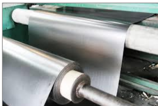
Figure 1 Expanded graphite and graphite foils produced from expanded graphite
