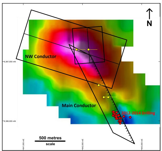
Figure 2–Zealous: Channel 25 MLEM Survey image with modelled conductor plates, historic drilling (red) and planned drilled (yellow)
