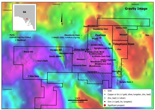
Figure 1 – Wilcherry Project plan showing location of MLEM surveying completed at Zealous and Telephone Dam. Background image is gravity
