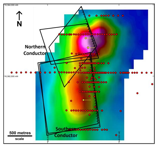
Figure 3—Telephone Dam: Channel 25 MLEM Survey image with modelled conductor plates, historic drilling (red) and planned drilling (yellow)
