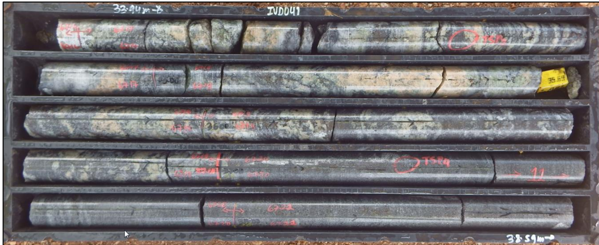
Figure 5: Example of migmatitic graphite gneiss (approximately 6% TGC) between 33.4 and 38.6 m downhole in IVD041
