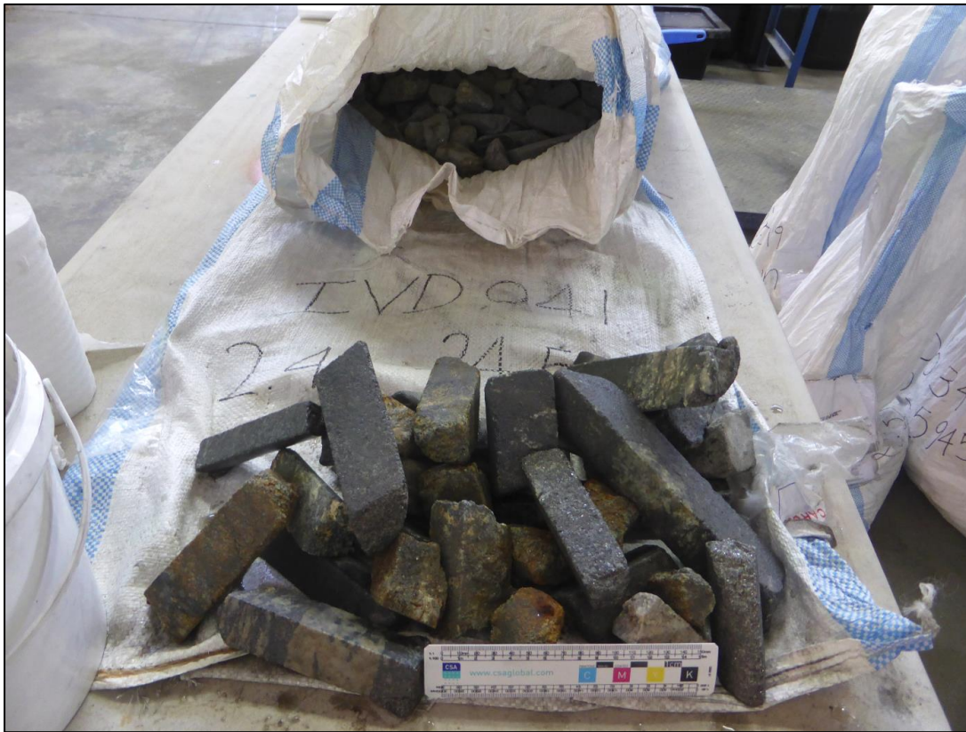
Figure 12: Example of quarter core samples submitted for metallurgical testing from IVD041 composite 12
