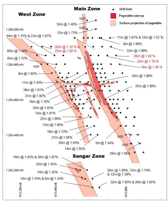
**Figure 1.** Goulamina Deposit. Plan view of lithium pegmatite with drill hole locations and selected drill intersections from Phase 2 program. Infill drilling intersections are excluded.
