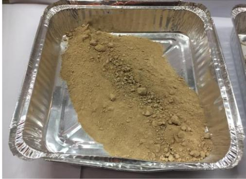
High-Phosphate Concentrate feed to the pilot plant
