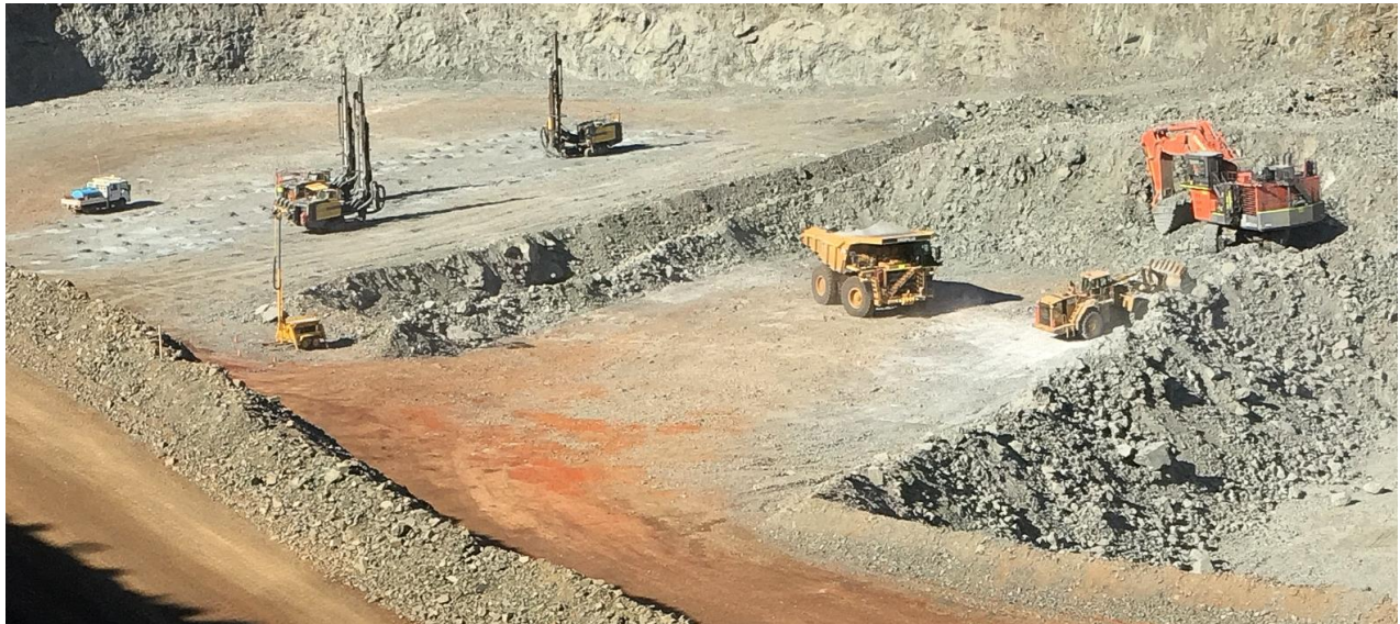
Figure 02: AEM mining chalcopyrite dominated ore (primary sulphide ore) in the south of the LM2 pit, whilst blast-holes for the next mining sequence are drilled in the background.
