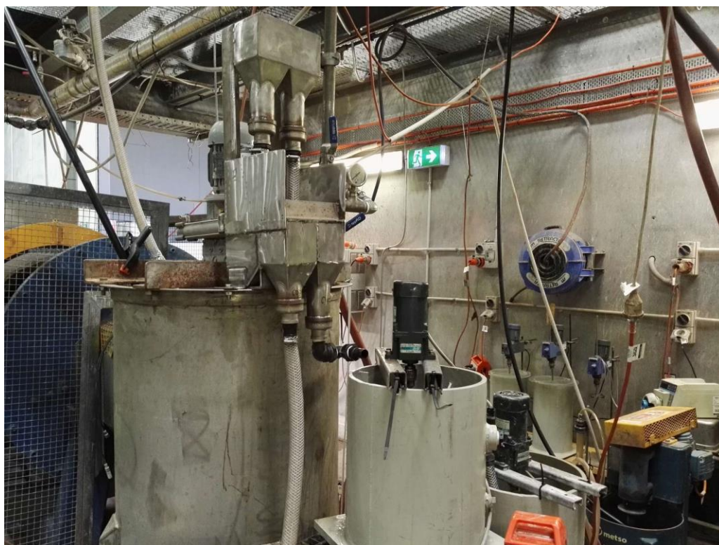
Figure 5: Flotation Pilot Deslime and Conditioning
