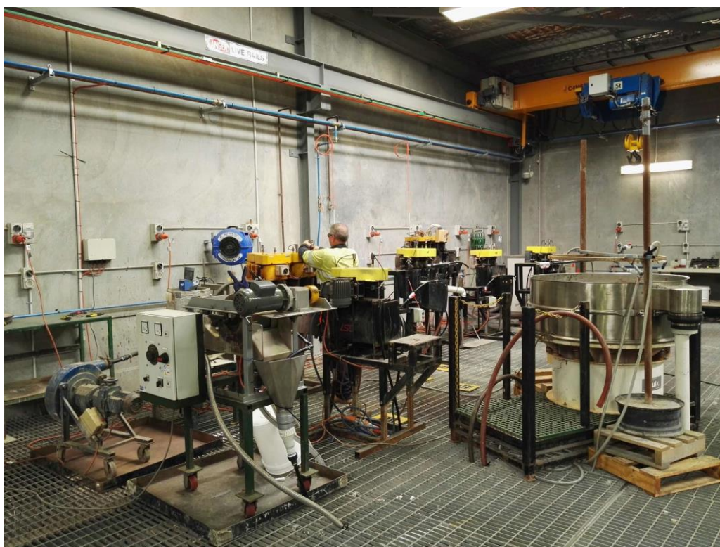
Figure 6: Flotation Pilot Low Intensity Magnetic Separation (LIMS), Screening and Flotation
