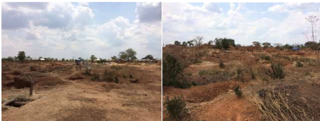
Figure 3 & 4 Artisanal workings at Uyowa targeting quartz veins within the shear zone hosted gold deposit.
