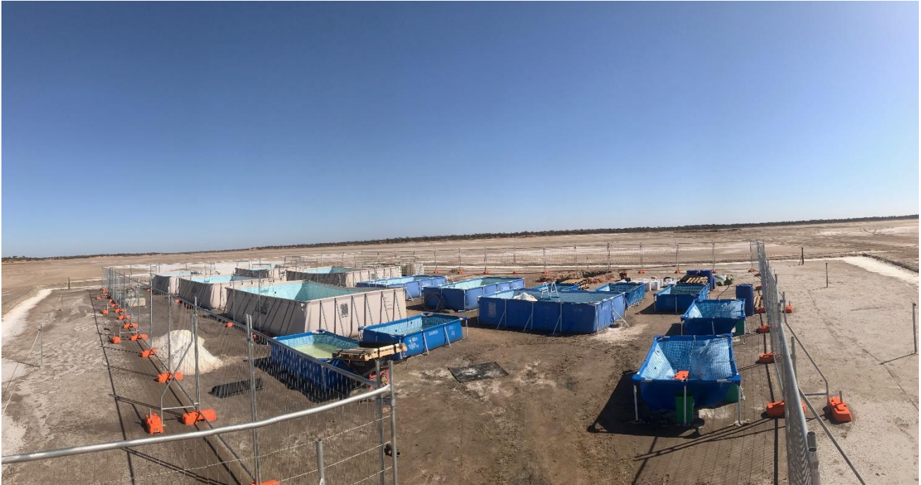
Figure 4: Site Evaporation Trial with Two Pond Trains in Operation
