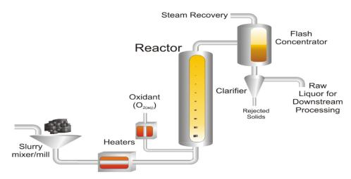
For lignite and lignin most the material is chemically converted [the OHD process] with a reaction time of less than a minute. The output from the reactor is a liquid which is about 98.5/99.5%% water, and 1.5/0.5% by weight organic chemicals in solution (the bio-stimulant fertiliser).
