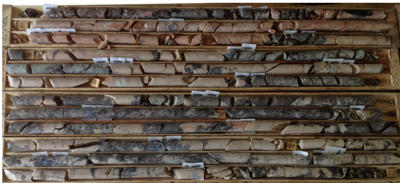
Figure 1. Drill core from diamond drill hole SL-17-02 showing high quality spodumene mineralisation from 0m to 17m.
