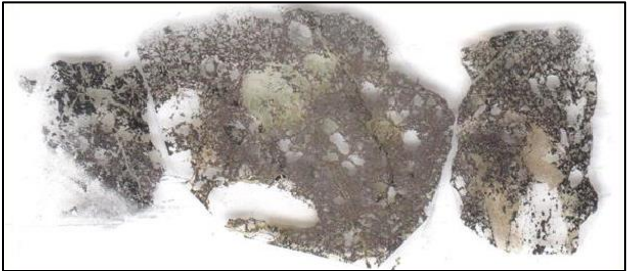
Polished thin section – dark and brassy domains are sulphides
