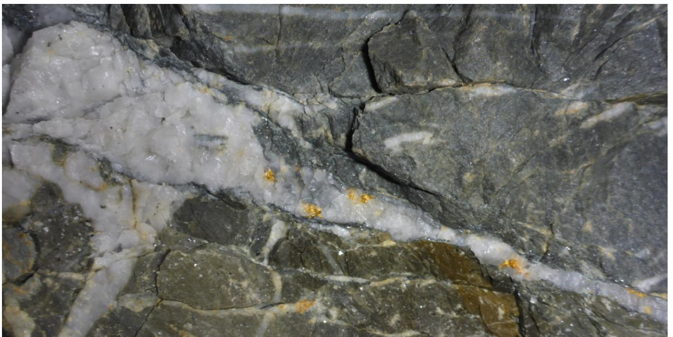
Figure 13. Image of free gold in face of 1465-8764 Airleg Stope at the A1 Mine
