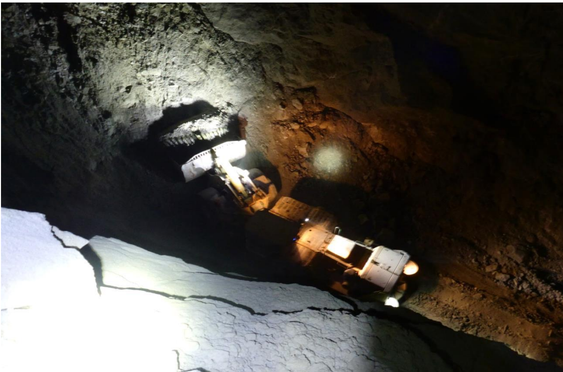
Figure 8. View from 1394 Level of the Tele Remote Control Bogger loading Ore in the Long Hole Stope on the 1380 Level at the A1 Mine
