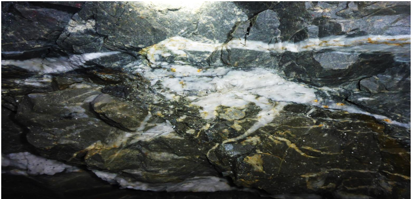
Figure 12. Image of free gold in face of 1465-8764 Airleg Stope at the A1 Mine
