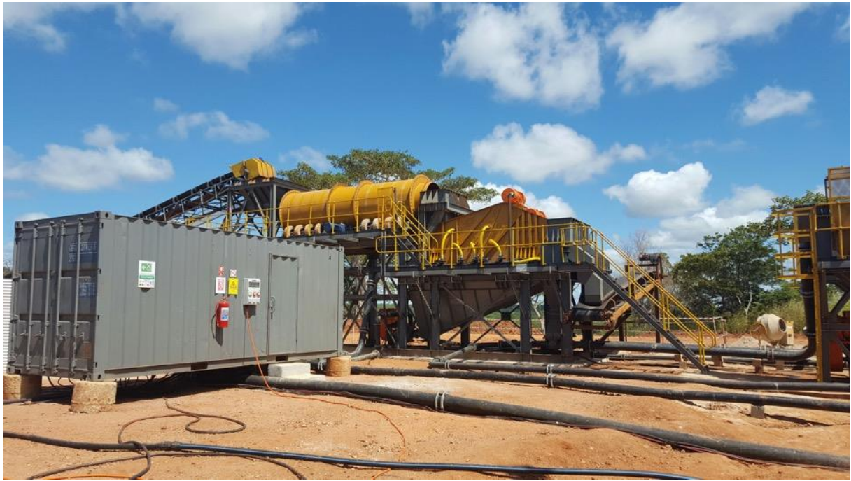
Figure 1. New wet-front end & upgrades of Mustang bulk sampling processing plant
