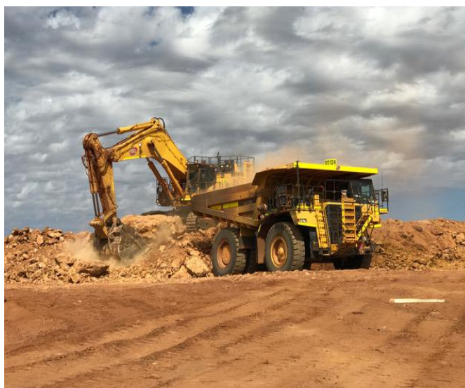
Photo 1: Digging first bench at Galaxy pit.
