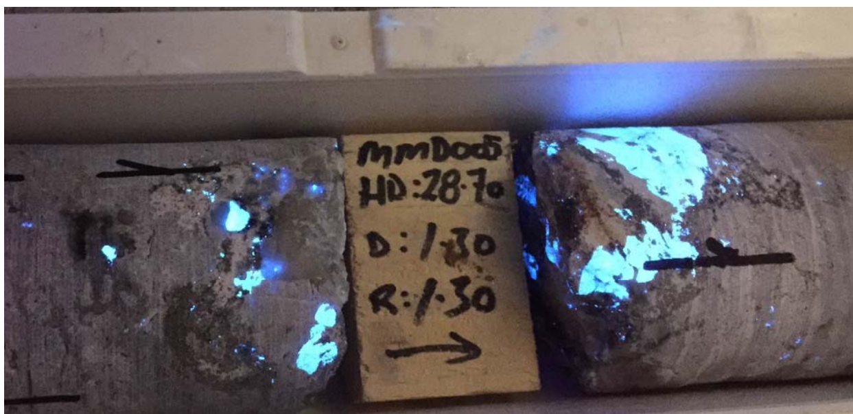
Figure 6: Diamond core from August 2016 drilling program showing course grained scheelite under UV
